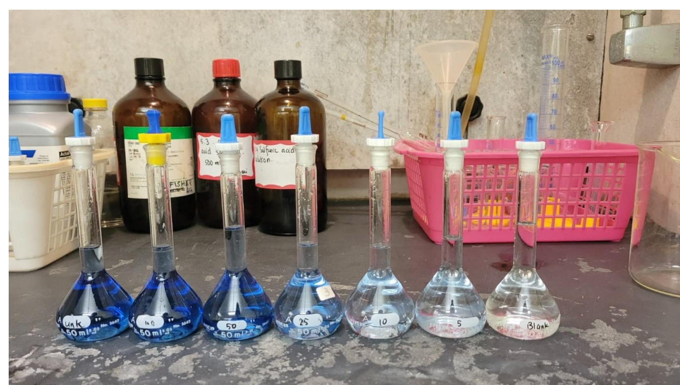
Figure 6: Standard solution with blue color from highest concentration of Silicate (left) to lowest concentration of Silicate (right)
