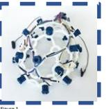
OPENBCI's **UltraCoretx Mark IV** is an open-source, 3-D printable headset that uses 16 dry electrodes, spatially distributed over the scalp in the 10-20 system of electrode placement, to acquire the oscillations of brain electric potentials. This headset is capable of recording research-grade brain activity
